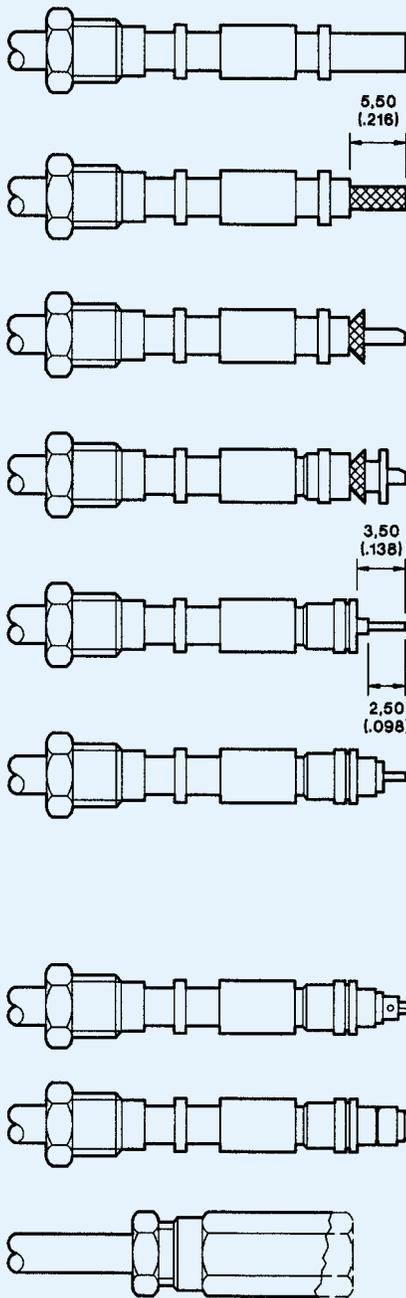
1. Slide clamp nut, No. 1 washer, gasket and No. 2 washer over cable.
