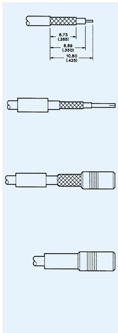
1. Trim cable to dimensions shown. Do not nick outer braid or center conductor. Tin center conductor with solder (DO NOT OVER TIN).
