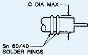
2. Place two solder rings per table below, over the cable.
