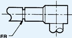
4. Push cable into body and solder in place.
