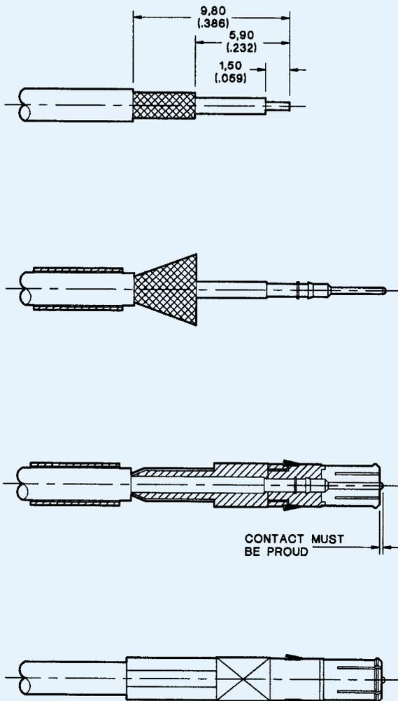
1. Trim cable to dimensions shown being careful not to nick or damage braids or center conductor. Twist center conductor filaments together.
