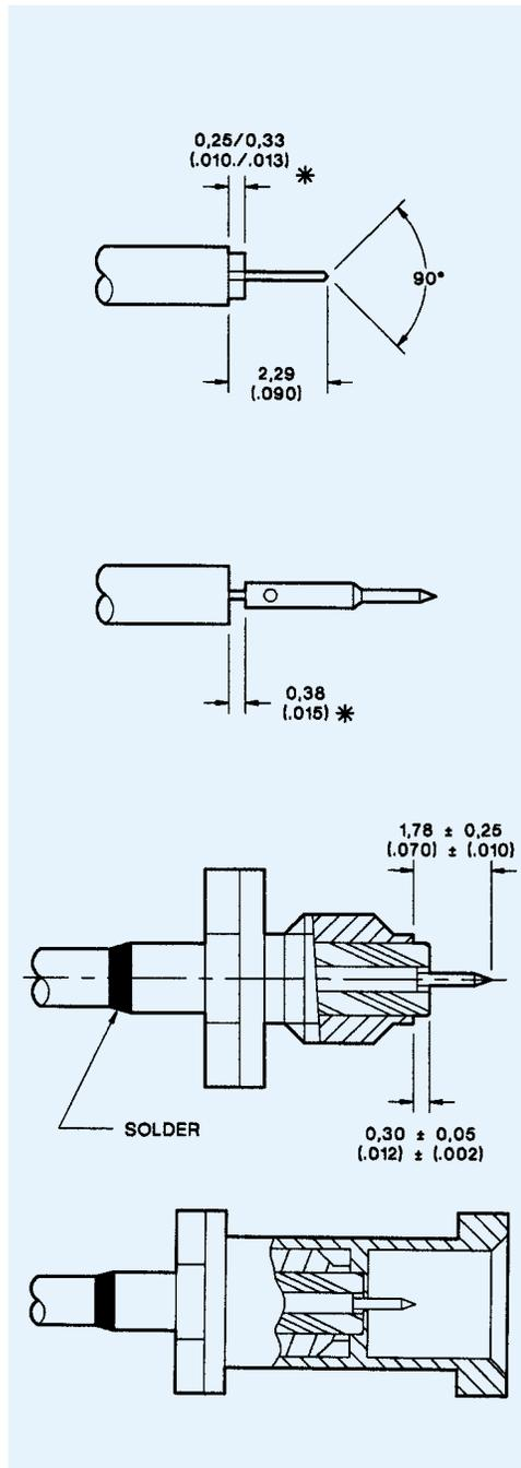
1. Trim cable to dimensions shown, being careful not to nick center conductor. Tin center conductor (DO NOT OVER TIN).
