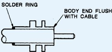
4. Clean housing area of outer conductor with abrasive paper and clean in a suitable agent. Place 24 s.w.g. soldering ring and connector body on prepared end of cable. Ensure body is correct way round. End of cable to be flush with end of connector body as shown.
