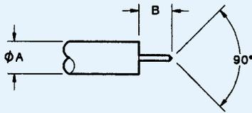
1. Trim cable to dimension 'B' shown. Being careful not to nick the center conductor.
