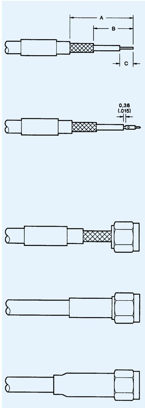
1. Trim cable to dimensions shown being careful not to nick the braid or center conductor. Tin center conductor, (DO NOT OVER TIN) then slip ferrule (and shrink tubing if supplied) over cable.
