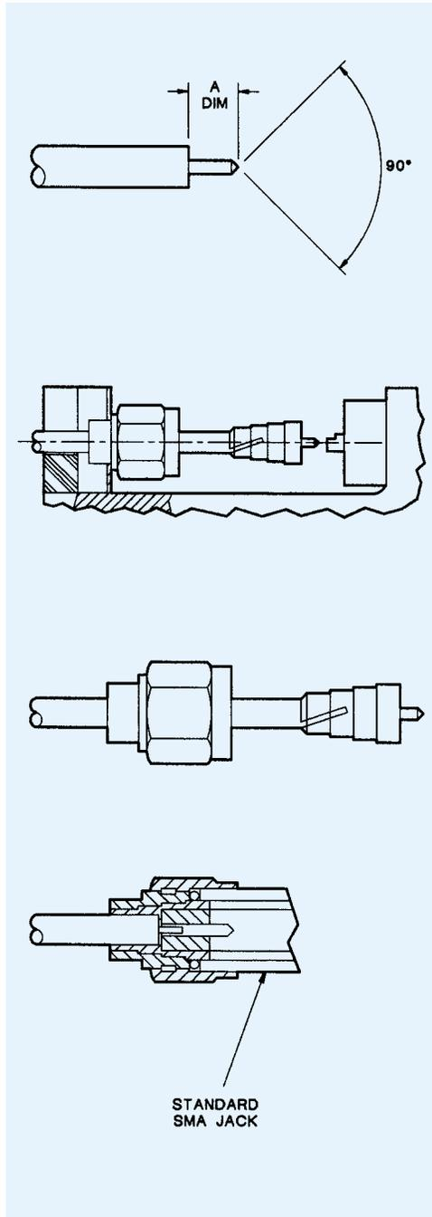
1. Trim cable to dimensions shown. Be careful not to nick center conductor. Ensure dielectric is flush. Remove burrs from the copper jacket end. Pointing of the center conductor is essential.
