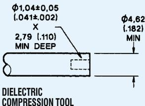
5. Compress expanded dielectric back into cable outer conductor with Dielectric Compression Tool as shown, until it is flush with end of body and outer conductor.
