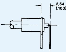
4. Bend center conductor to dimension shown depending upon preferred orientation. These dimensions suit 2,54 (.100) and 7,62 (.300) PCB pitches. For other pitches of 2,54 (.100) multiples add 2,54 (.100) multiples, to the 12,70 (.500) and 6,35 (.250) dimensions in the cable stripping instructions Note 1.
