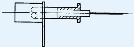
3. Slide tab-ferrule over braids to face of flange and crimp using ITT Cannon crimp tool and suitable die set (see table).
