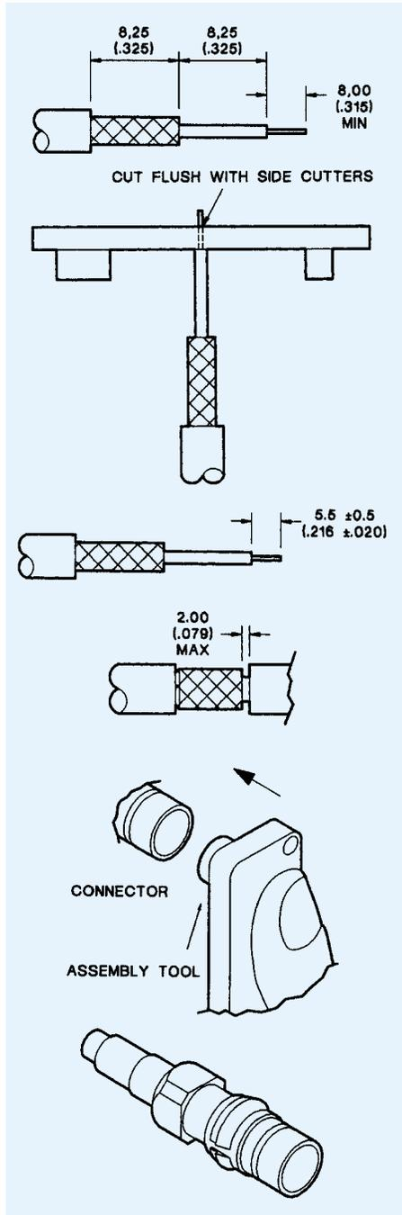
1. Prepare cable, using a suitable stripping, tool to the dimensions shown being careful not to damage the braid, dielectric or inner conductor.
