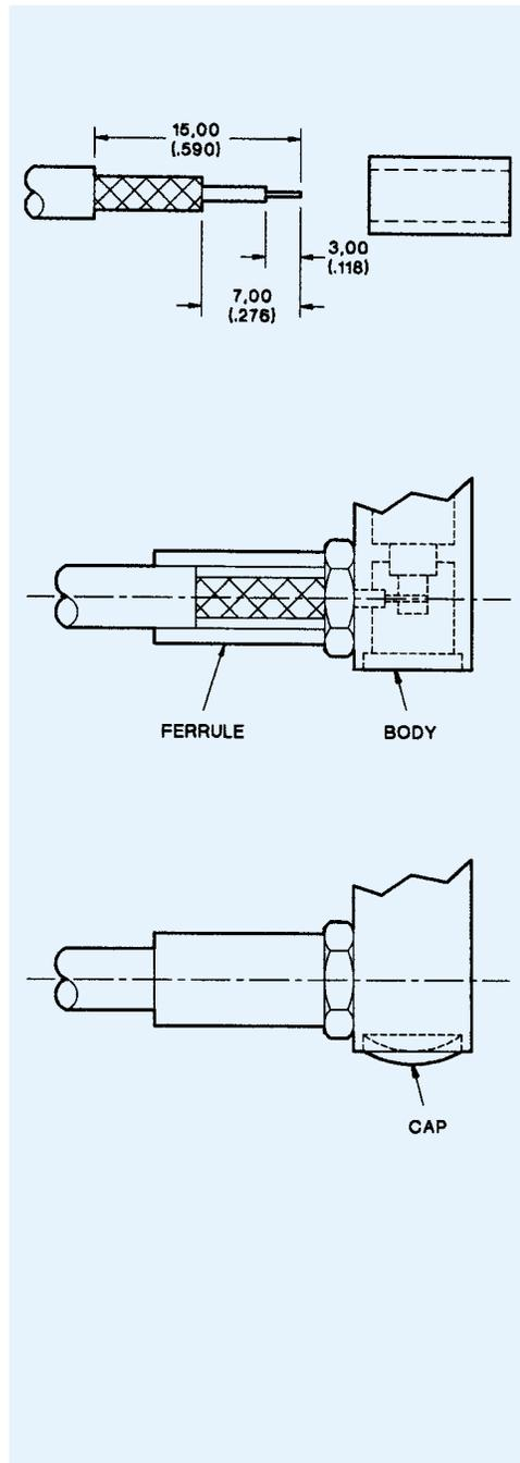
1. Trim cable to dimensions shown being careful not to nick the braid or center conductor. Tin center conductor, (DO NOT OVER TIN), then slip ferrule over cable.
