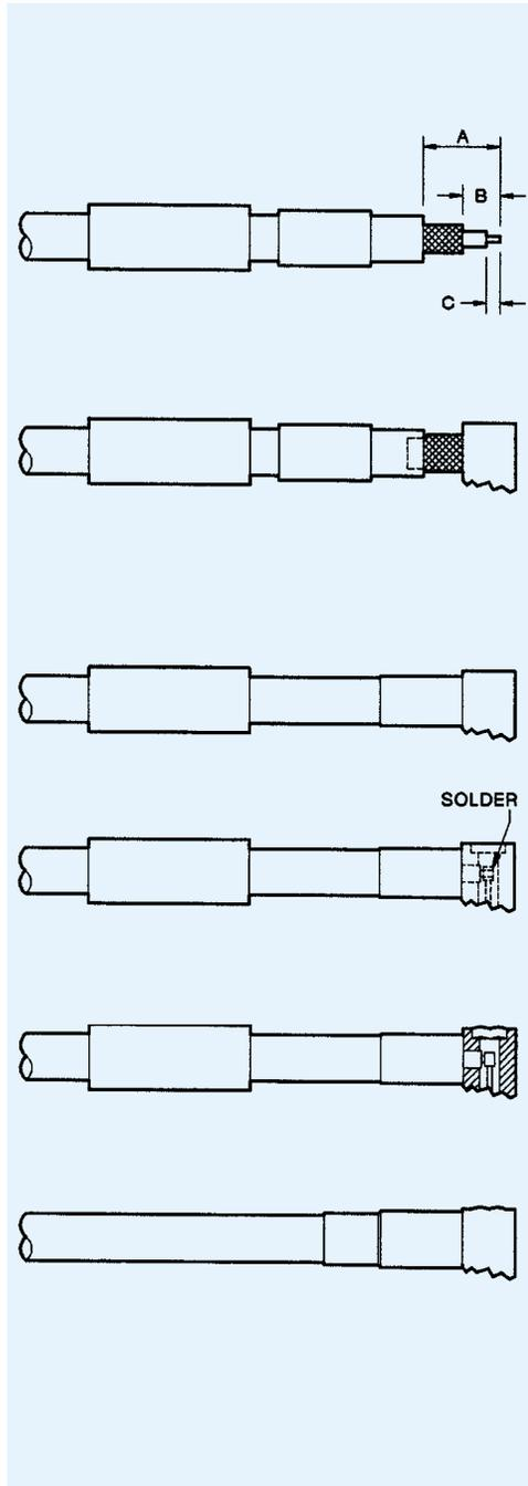
1. Slide heat shrinkable tubing and ferrule on to cable.
