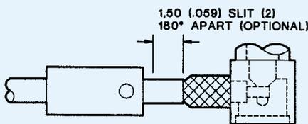
2. Insert trimmed cable into back end of body. The tubular body extension will slide under the braid with the rear portion of extension fitting under the jacket as shown. The center conductor will extend into slot in contact.
