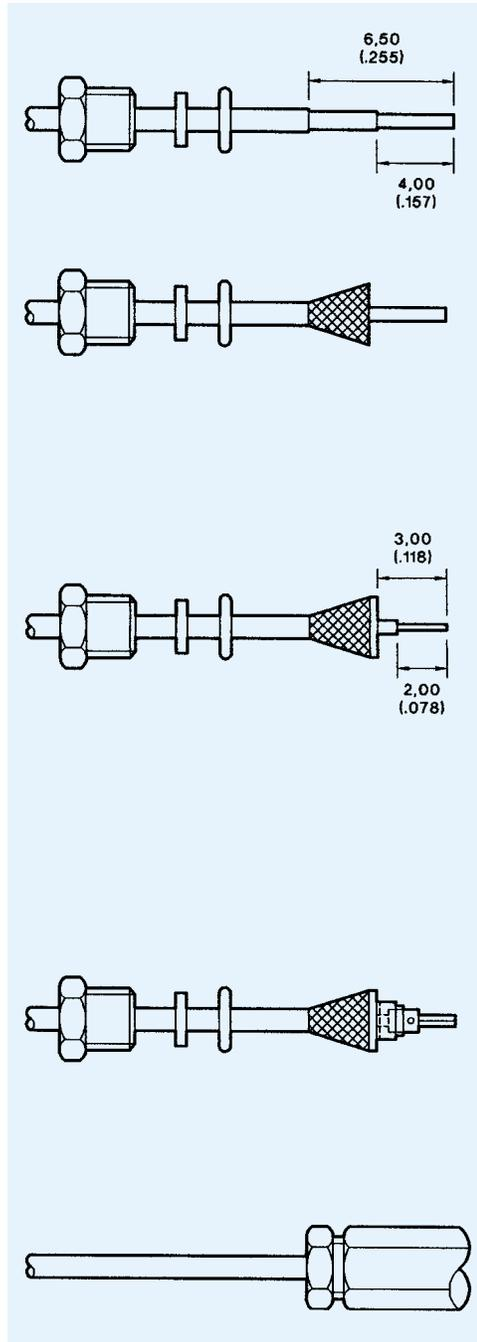
1. Slide clamp nut, washer and 'O' ring over cable.
