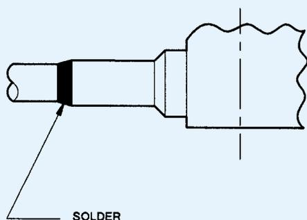
2. Insert cable into rear of body until cable seats in counterbore. Holding firm in this position. Solder cable to body.
