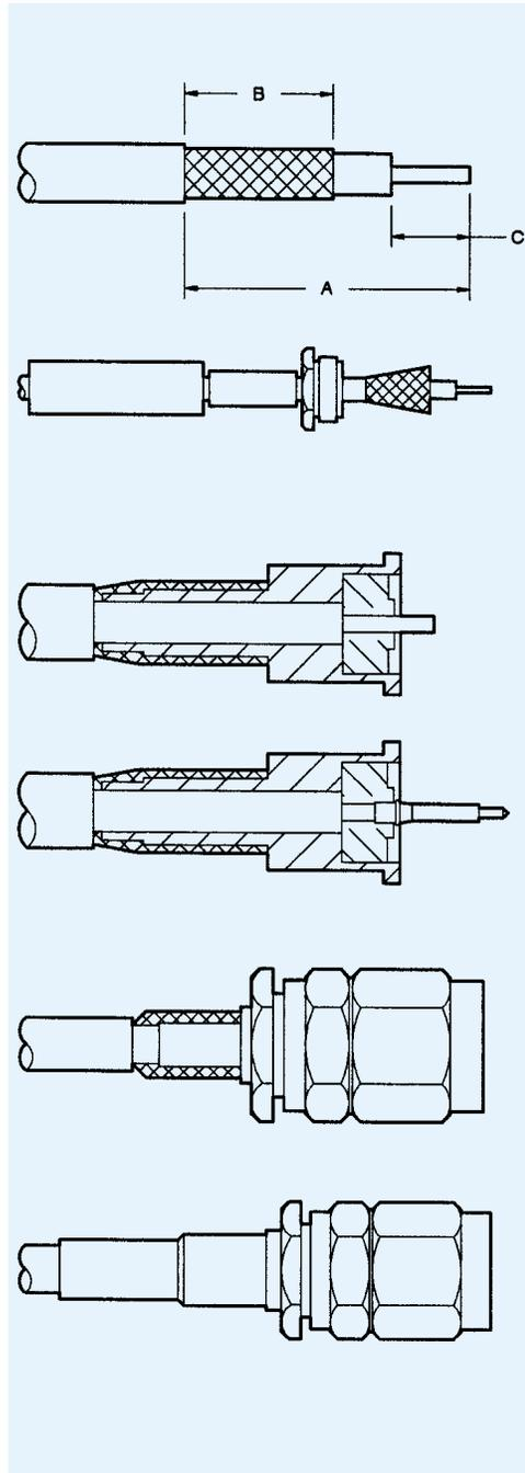
1. Strip cable to dimensions shown. Do not nick outer or inner conductors. Tin inner conductor.
