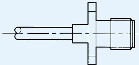
3. Slide contact and cable into rear of body assembly until it seats firmly against insulator in body. Solder cable to body applying sufficient heat to body for solder to flow, but using minimum heat cycle.
