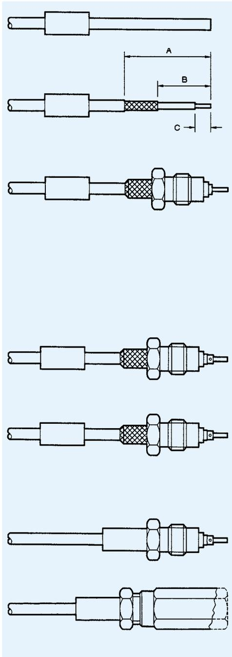
1. Slide ferrule on cable, (and tubing with SMS)
