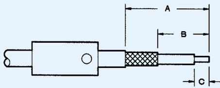
1. Trim cable to dimensions shown taking care not to nick braid or center conductor. Tin center conductor (DO NOT OVER TIN) then slip crimp ferrule (and tubing with SMS) over cable with inspection hole toward trimmed end.
