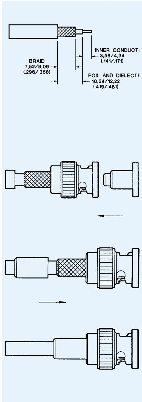
1. Prepare cable using a suitable stripping tool to the dimensions shown, being careful not to damage the braid, dielectric, foil or inner conductor.
