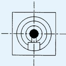
3. Orientate slot of contact and insulator to be parallel to the cable entry hole as shown.
