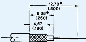
1. Trim cable to dimensions shown being careful not to nick or damage braids or center conductor. Trim center conductor.
