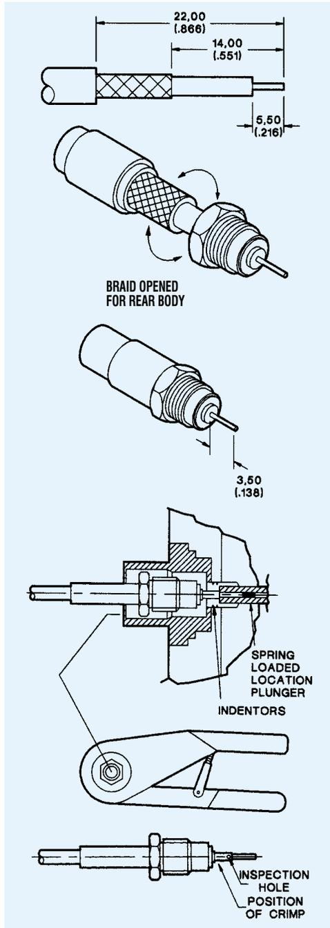
1. Check that the center contact is a free fit in the front insulator and that you have all the connector parts. The termination technique and cable preparation dimensions for the sockets are the same.
