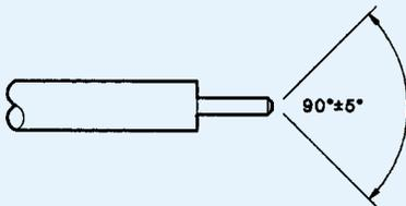
2. Point the end of the center conductor using Tool T2297 if available or a miniature file.
