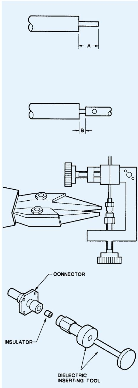
1. Cut cable end square. Trim the cable outer conductor and dielectric as shown taking care not to nick the center conductor. Deburr outer conductor at point of cut.
