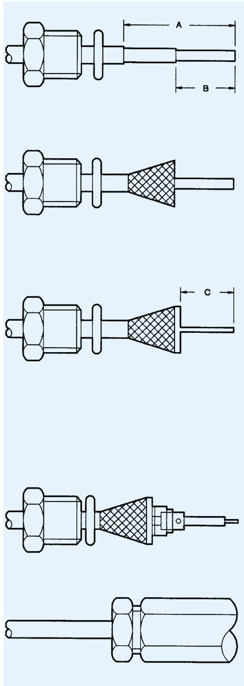
1. Slide clamp nut and 'O' ring over cable.
