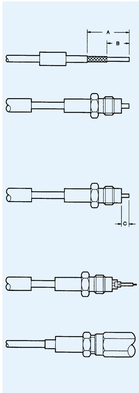
1. Slide ferrule and heat shrinkable tubing on to cable.
