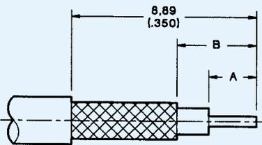
1. Dip 9,50 (.374) to 12,70 (.500) of both ends of the cable into a solder pot. Flux may be applied to the ends of the cable prior to dipping, if desired.
